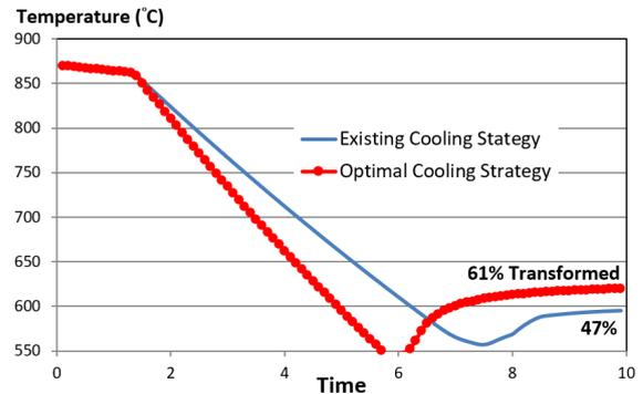
Fig.7. Optimal cooling strategy for medium carbon steel.
