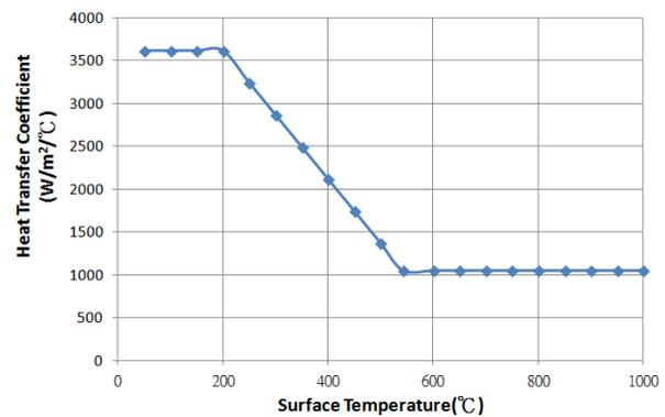
**Fig.2.** Heat transfer coefficient for the water cooling.
